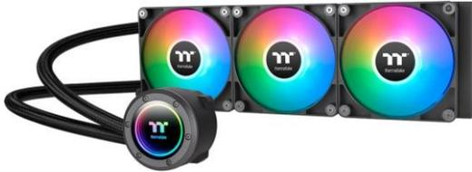
Lüfter: 3x 120mm, Material: Aluminium, TDP: k.A. Intel Socket 1700, 115x/1200, 1356/1366, AM2/AM2+/AM3/AM3+, AM4, FM1/FM2/FM2+
